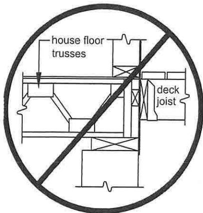
**FIGURE 17: FLOOR TRUSSES**
