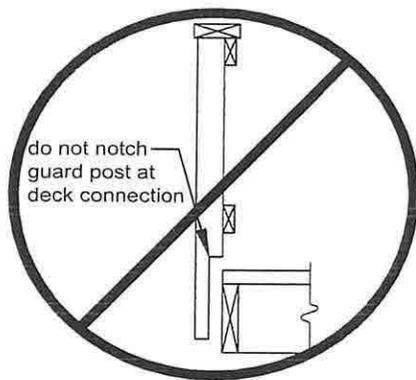
**FIGURE 28: NOTCHING AT GUARD POSTS**
