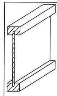
**FIGURE 13: WOOD I-JOIST PROFILE**
