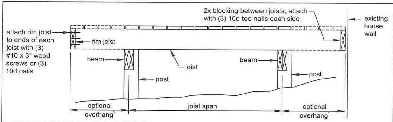
**FIGURE 4: JOIST SPAN - FREE-STANDING DECK<sup>2</sup>**
