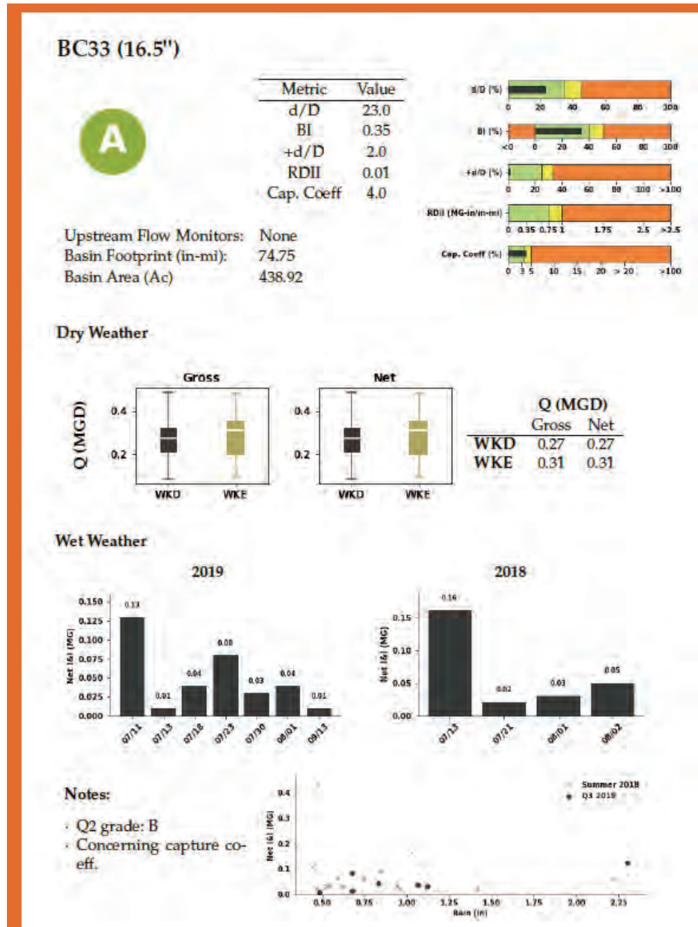
Report Card Produced by Python software to make comparisons in wastewater collection system flow monitors for year and seasons.
